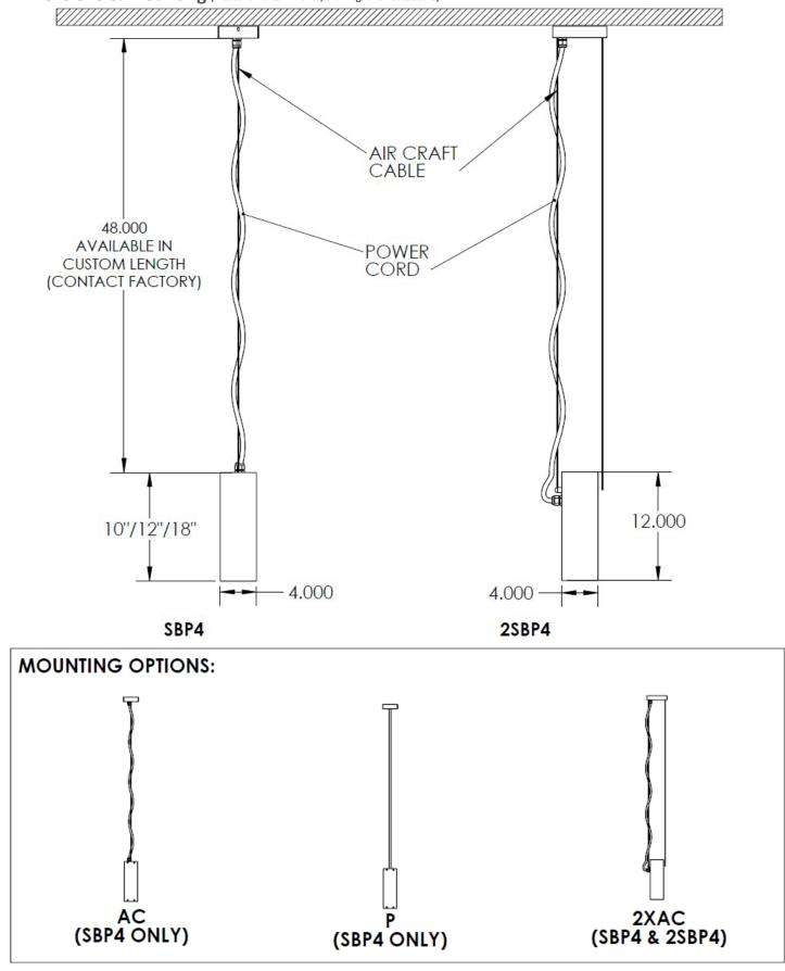
Dimensions & Mounting (measurements in inches; drawings are not to scale)
