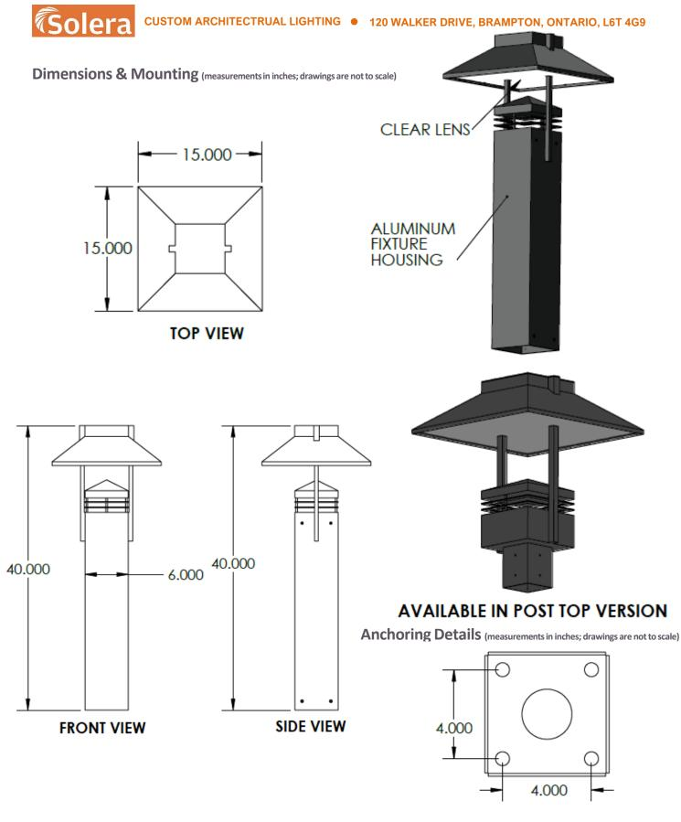
Anchorbolt Size: 1/2" X 12" X 1-3/8" -Hot dipped Galvanized anchor bolts -Galvanized steel hex nuts -Galvanized steel flat washers
